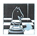
The pattern was directly written in a resist by electron beam lithography using the ZBA 23H from Leica Microsystems Lithography GmbH, and pattern transfer in the gold layer was done by ion beam etching.
